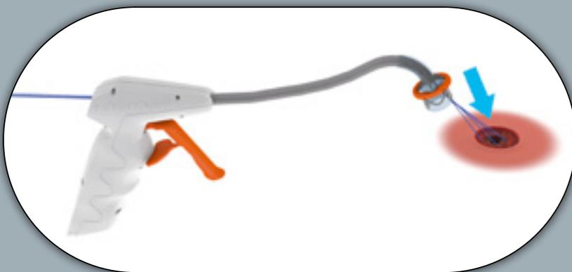
The designated application site for the clip is lined up with the application cap which is pressed on the target site. To facilitate this procedure two U-shaped sutures can be placed through the sphincter muscle centering the internal opening of the fistula in a cross-like fashion. The ends of the threads are pulled through the working channel of the instrument by means of the thread retriever.
